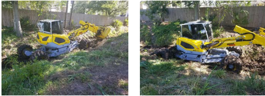
Images of Menzi Muck cleaning vegetation from the B-7E canal.
