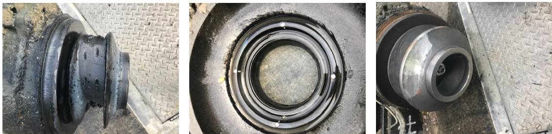
Images of wear rings on lift station.
