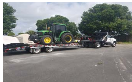
Image of new 20-ton trailer and Ford F-750 dump truck transporting the John Deere mower.
